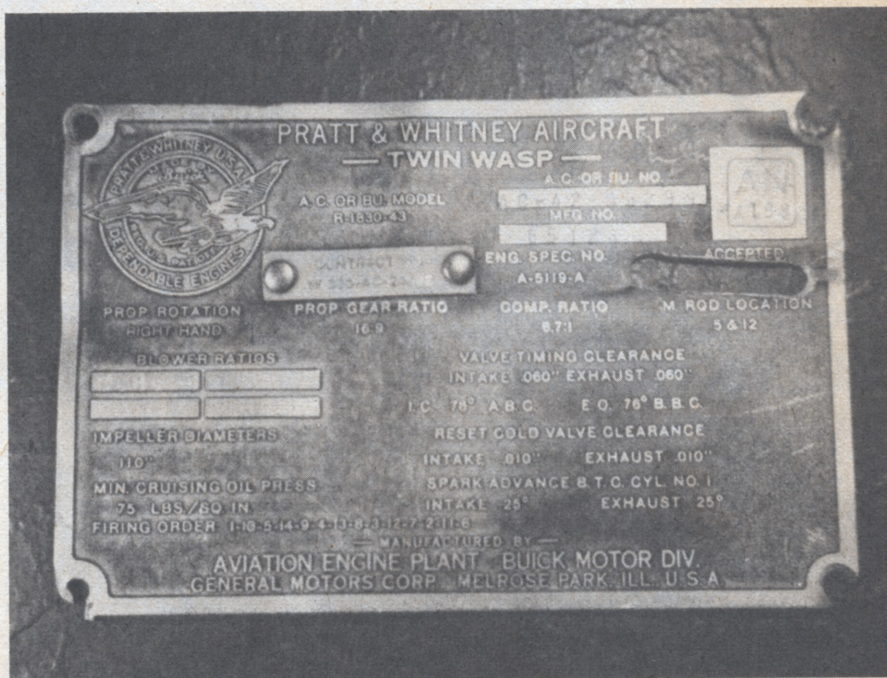
Number 4 engine identification plate buried in the desert sands for 26 years was the major clue that revealed the full story of the Hammer Field B-24 mishaps during December 1943.
