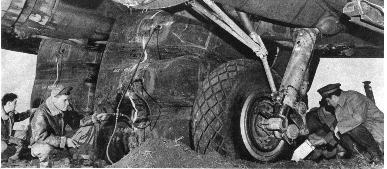
4 Huge balloon jacks, inserted flat between inboard engines and fuselage, raise Sir Baboon's 40,000-odd pounds easily. Wheels and other parts of plane's underside are checked carefully for damage. Note unusual bomb rack under wing close to fuselage.
