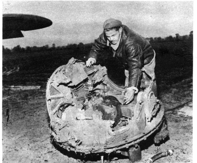
6 The belly turret bore brunt of the landing and sections of it shattered off on impact. The gunner was not in it.
