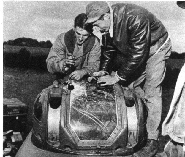
8 Damage to turret was result of a 20-mm. cannon hit by a Focke-Wulf Fw-190 during plane's mission over Germany.
