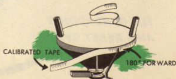
PUT A PIECE OF EXPOSED FILM IN SIGHT TO LOOK AT SUN READ BEARING OFF STATIONARY RING
