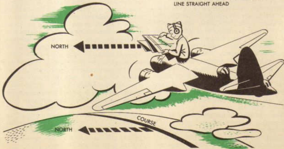
ORIENT MAP BY ALIGNING COURSE LINE STRAIGHT AHEAD
