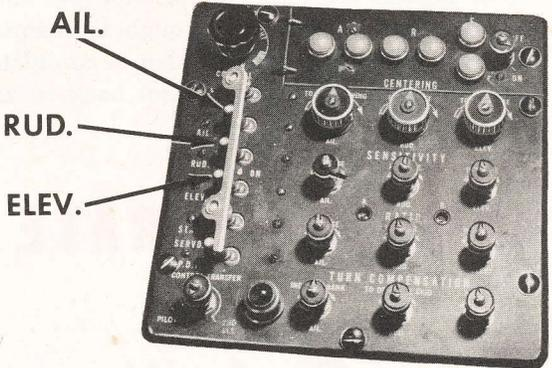
6. Make final autopilot trim corrections. If necessary, use centering knobs to level wings and center PDI.
