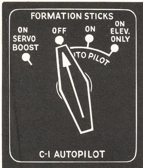
2. "ON SERVO BOOST"—The stick is in direct control of the autopilot servos and you must use it as if it were mechanically linked to the surface controls. Use this position when you want quick maneuvering, as in a wing position of a tight formation.
