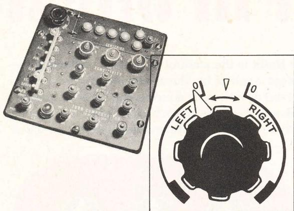
The **turn control** is used by the pilot to turn the airplane while flying under automatic control. To adjust turn control, first make sure turn compensation adjustments have been properly made, then set turn control pointer at beginning of trip-lined area on dial. Airplane
