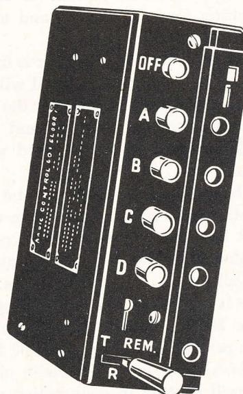
to transmit. In the "T" position the transmitter is in continuous operation. In the "R" position the receiver is in continuous operation.
