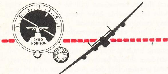
should bank 30°, as indicated by artificial horizon. If it doesn't, remove cap from aileron trimmer and adjust trimmer until a 30° bank is attained. Then, if turn is not coordinated (inclinometer ball not centered), adjust rudder trimmer to center ball. Make final adjustments with both trimmers and replace caps. Set turn control at zero to resume straight and level flight; then re-center.
