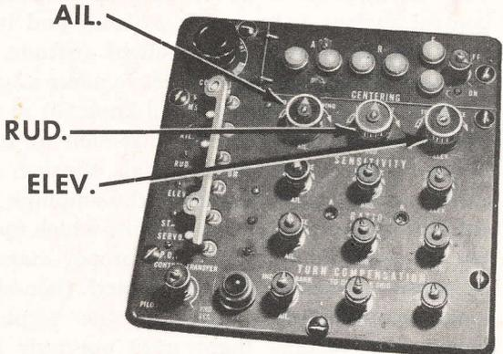
5. Engage the autopilot. Put out aileron tell-tale lights with the aileron centering knob, then throw on the aileron engaging switch. Repeat the operation for rudder, then for elevator.
