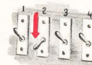
9. **Generator Off.** Engineer switches off generator on dead engine.
