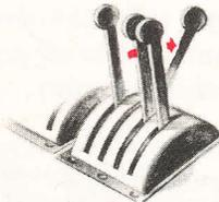
3. **Mixture and Fuel Booster Pump.** Copilot moves mixture control to "IDLE CUT-OFF" and switches fuel booster pump off. This is necessary at times to stop the engine.
