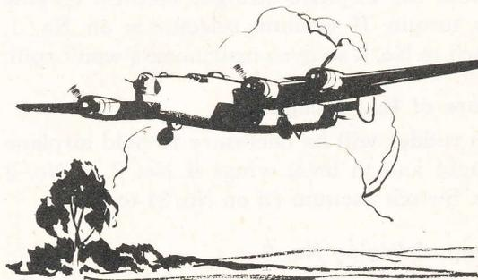
4. Get and keep control with rudder and minimum aileron. Insufficient rudder and too much aileron will put you in a forward slip and you
