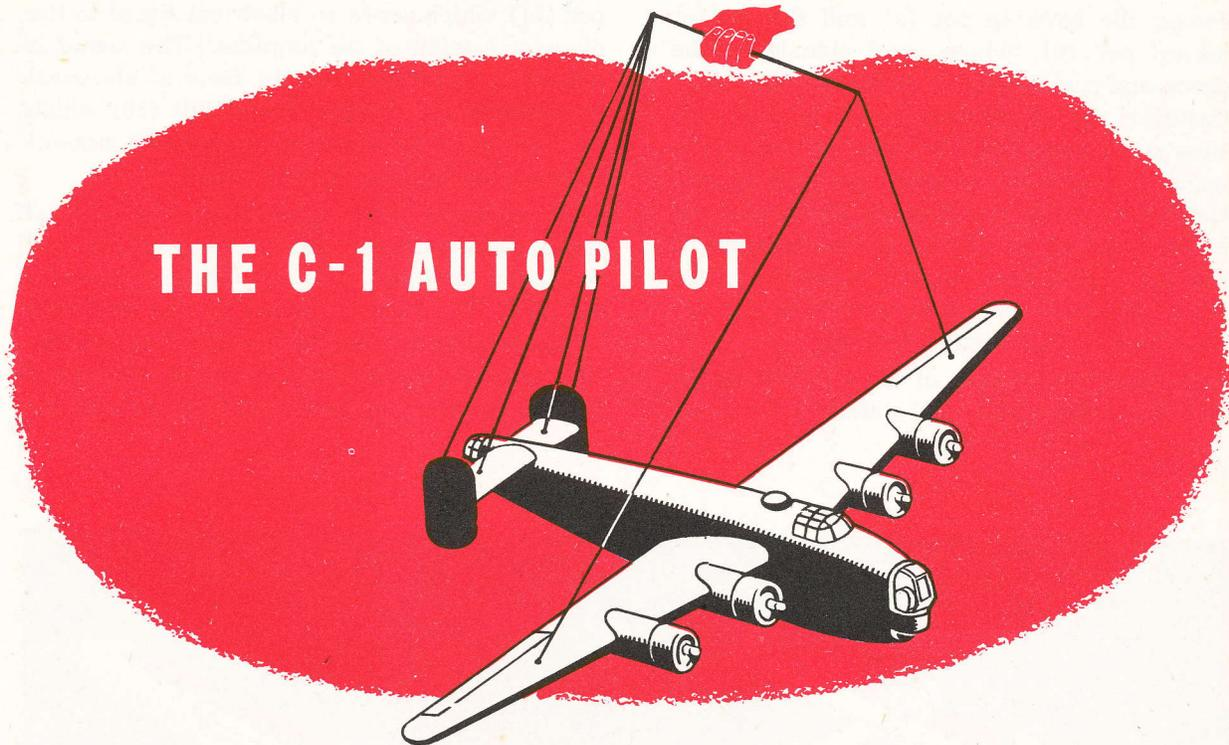
The C-1 autopilot is an electromechanical robot which automatically controls the airplane in straight and level flight, or maneuvers the airplane in response to the fingertip control of the human pilot or bombardier.
