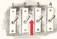
**9. Generator On.** When power is increased as engine warms up generator is turned on.
