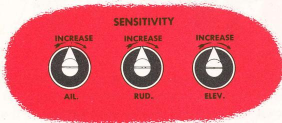
**Sensitivity** is comparable to a human pilot's reaction time. With sensitivity set high, the autopilot responds quickly to apply a correction for even the slightest deviation. If sensitivity is set low, flight deviations must be relatively large before the autopilot will apply its corrective action.
