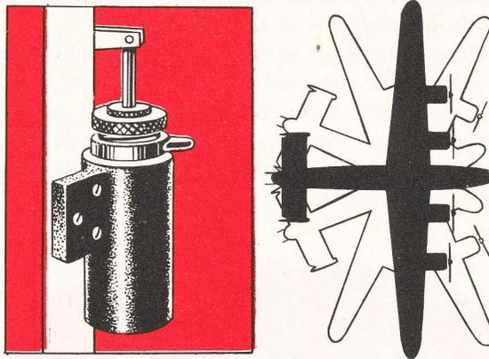
This is accomplished by loosening the locknut on the dashpot, turning the knurled ring up or down until hunting ceases, then tightening the locknut.
