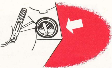
4. Have the bombardier disengage the autopilot clutch, center PDI and lock it in place by depressing the directional control lock. The PDI is held centered until the pilot has completed the engaging procedure. Then the autopilot clutch is re-engaged, and the directional arm lock released.
