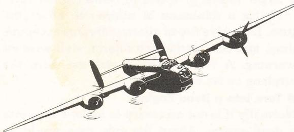
Normally, with one engine dead, maximum cruise power settings will easily maintain level flight. When the engine first fails, you may want to use maximum climbing power and, in combat, danger from the enemy or maintaining position in formation will govern your actions. But don't pour the power on unreasonably. Second and third engine failures too often are induced by using power improperly. Handle
