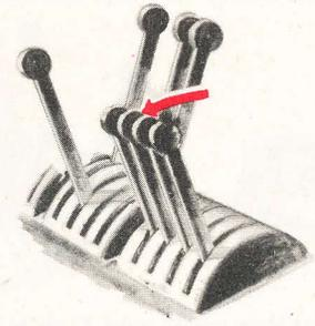
**7. Mixture Auto-rich.** Copilot puts mixture control in "AUTO-RICH," booster pump off.
