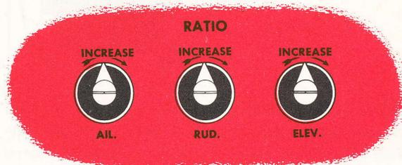
If ratio is too high, the autopilot will overcontrol the airplane and produce a ship hunt; if ratio is too low, the autopilot will undercontrol and flight corrections will be too slow. After ratio adjustments have been made, centering may require readjustment.
