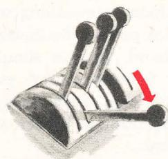
**5. Supercharger Off.** Pilot checks to see that supercharger control is in off position (with oil regulated supercharger only).
