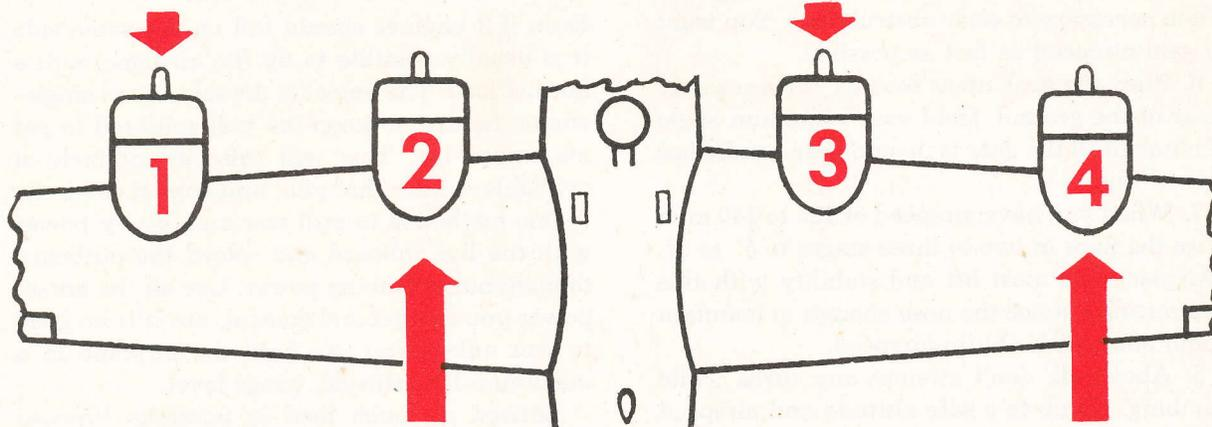
**No. 2 Dead**—You lose generator, heaters (for pilot, copilot and top turret gunner) and vacuum pump. Switch vacuum to No. 1.
