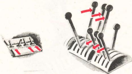
4. **Application of Power.** Copilot adjusts mixture controls on other engines and increases rpm. Pilot increases manifold pressure. Actions of pilot and copilot are approximately simultaneous, but the increase of mixtures and rpm should always precede the increase in manifold pressure.
