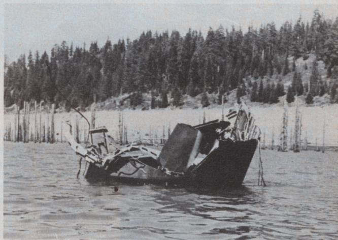
The B-24 broke into three pieces on impact. This is the forward part of the bomber. It broke off at the rear of the bomb bay. In this photo, the nose of the aircraft is buried in the mud. (L. D. Martin)
