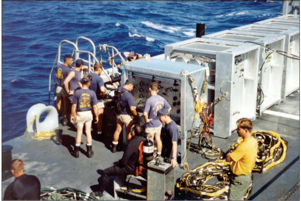
Figure 13-5. FADS III Mixed Gas System (FMGS).
