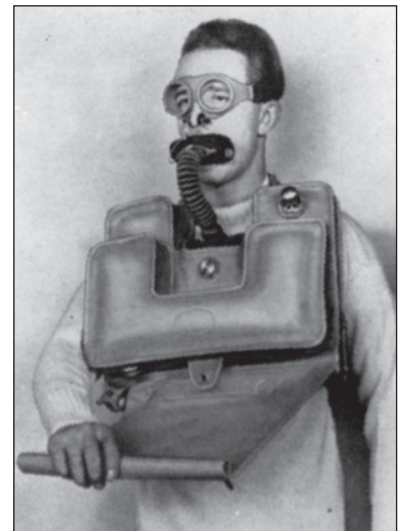
Figure 1-10. Original Davis Submerged Escape Apparatus.
